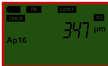
In the **memory mode** (**MEMO**) the measurements are not only displayed but also stored in different blocks. The display of the mean-value refers here always to the measurements that are currently stored in the active measurement block.
