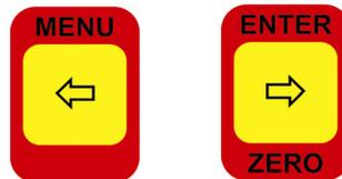
pushes the cursor on the device display according to the left or right. If you press the arrow keys **for more than 2 seconds** you can step quickly to the next input of scroll fast. For example, if you want to exceed the limit by 125  $\mu\text{m}$ , proceed as follows:
