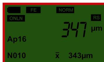
The active application (calibration of the probe) is shown in the figure after **Ap**. By pressing the button:
