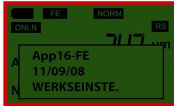
In addition to the basic point measurement (without storage), you can also perform **continuous surface measurements** (**CONT**) with this device. In this mode, two or three measurements are recorded and displayed within a second. However, please note that these measurements are not used to calculate the continuously determined mean value, so it will not be displayed. Online transfer of the data is not available in this mode either.
