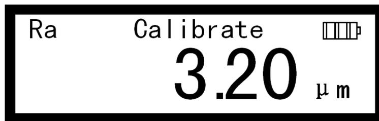
Using the arrow keys adjust the starting value to the value shown on the roughness standard.
