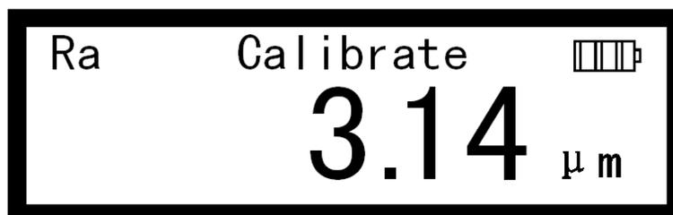
Put the instrument on the scribed line area of the standard and press the start button.
