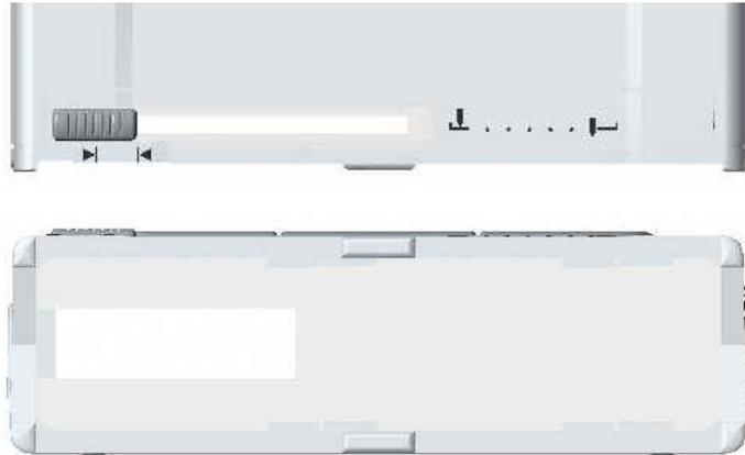
Move the switch to the right to open the protector so that the sensor comes out.
