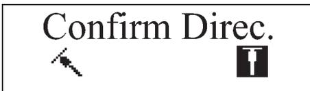
Both directions of and are different and need to be confirmed by hand. Press , to move the cursor to correct impact direction. Press to confirm. The indication of different direction displays is caused of shaking of impact device.
