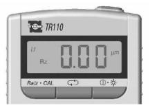
Press the Middle Key gently and quickly to select the sampling length (0.25mm, 0.8mm, 2.5mm) by turns. (Refer to Picture 5)
