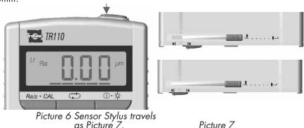
After two "di, di...." sounds, the measurement finishes, and the screen will show as the picture in the right.
