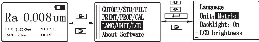
Figure 2-16 Metric/British system switching function
