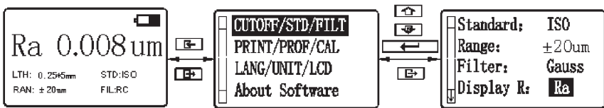
Figure 2-13 Modifying parameters to display
