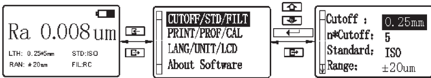
Figure 2-8 Select set measurement conditions status
