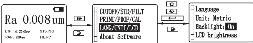
Figure 2-17 Back-light On/Off Function
